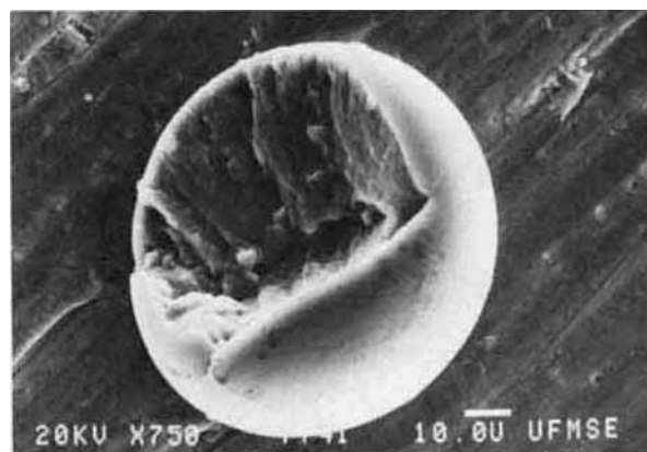
Figure 2—Scanning electron micrograph (750 \times ) of 100 \mu m albumin microsphere showing internal structure; polymethylmethacrylate dispersant.
