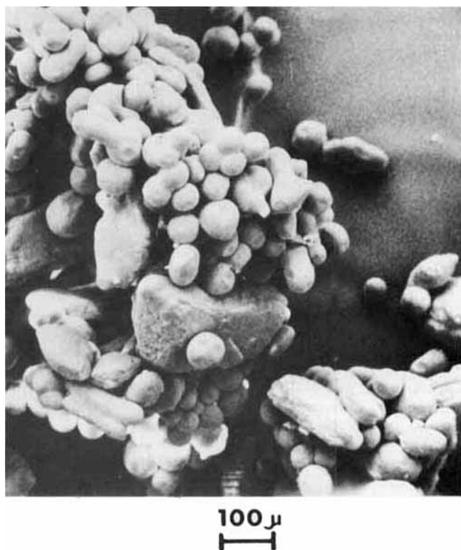
Figure 6 —Scanning electron micrograph of salicylamide microcapsules (250–300 \mu\text{m} ) with empty spherical coacervate droplets (40–60 \mu\text{m} ).
